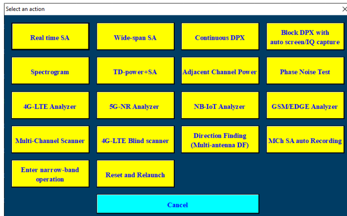
Figure 4 - Test selection menu dialog. The power and E-field switch is applicable to the 1 st row and first two tests at 2 nd row
