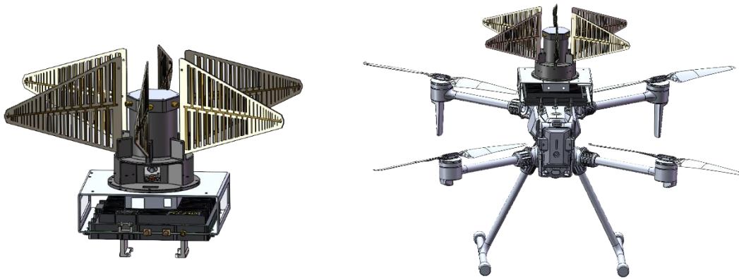
Figure 22, Left: the package containing a WSA-208 integrated with a 6-antenna-element; Right: such package mounted on a drone.
