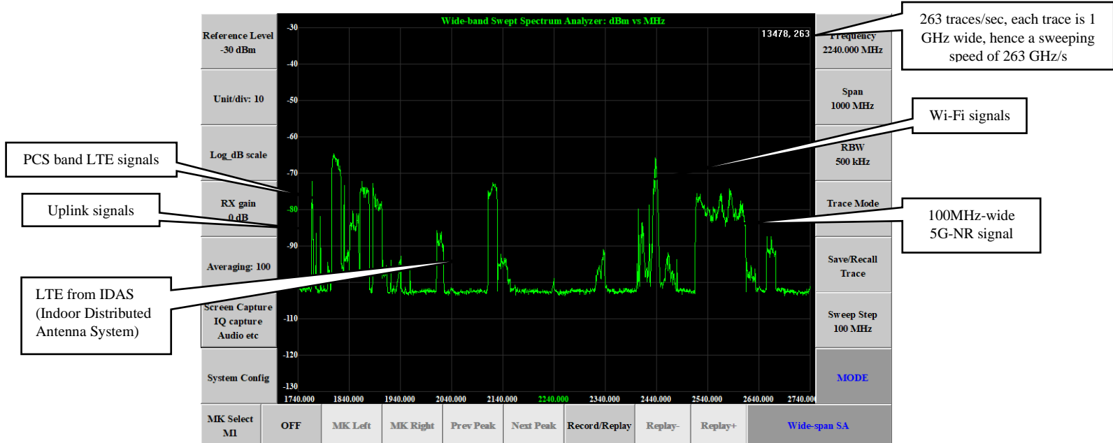
Figure 4, even in sweeping mode (span=1000 MHz here), the spectral display shows remarkable resolution for both amplitude and frequency and impressive interception of fast changing signals (TD-LTE, Wi-Fi and 5G-NR) without distorting their respective spectrum.
