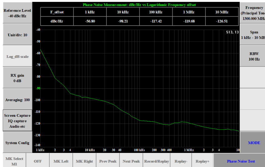
Figure 11, phase noise measurement example.
